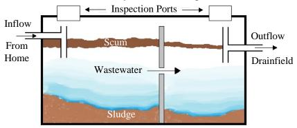
to the drainfield or individual lagoon. The tank will always be filled with liquid. Typically, when the sludge layer is over 2 feet high, it is time to have your tank pumped.
