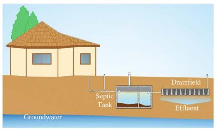
The second stage of treatment occurs when the effluent travels to the drainfield and distributes into the soil.
